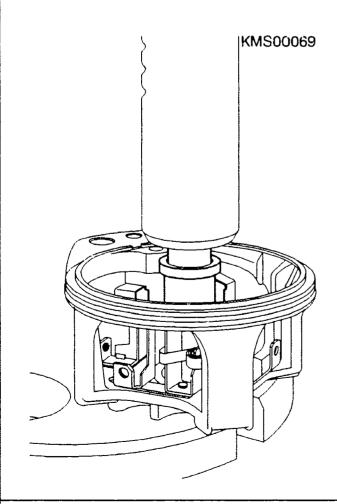
CHECKING AND REPAIRING COMPONENTS Checking commutator end shield Installation: Use reversed pressingout and pressing-in mandrel to press in new bushing. ATTENTION: Bushing must have been impregnated beforehand for 8 hours with Shell Tellus oil. Pressing-out and pressing-in mandrel for bushing in commutator end shield: 0 986 617 190
